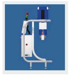
Bottom inspection to verify foreign bodies presence. Superior flange inspection to verify ovalizing, points and various defects.
